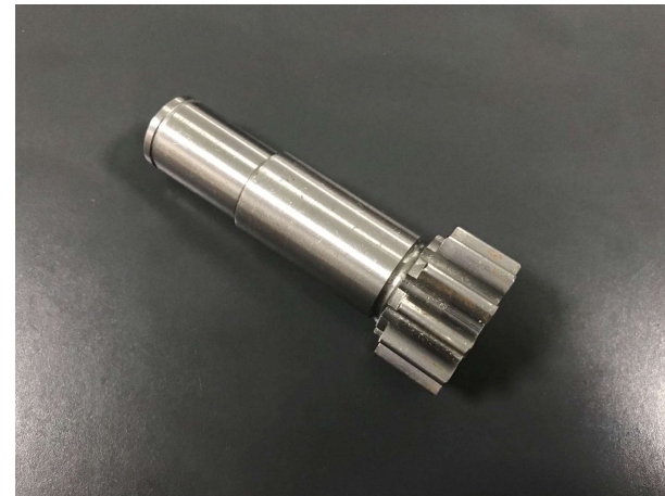
-Steel spur gear, -High Precision 0.005mm tolerance -Ra 0.3 -11 teeth
