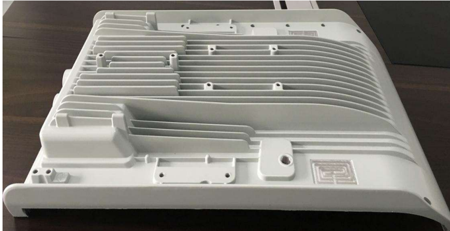
Aluminum Base Plate(57cm*45cm*31cm) 1600T Casting Machine
