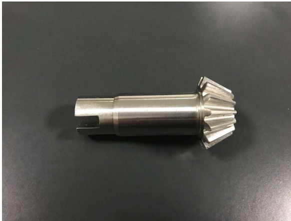
-SST Bevel Gear -High Precision 0.005mm tolerance -Ra 0.3 -15 teeth
